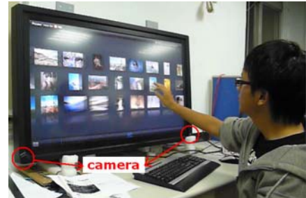
Fig. 7. An example of one finger touched the panel and our system drew a red point at where the finger touched on the screen.
